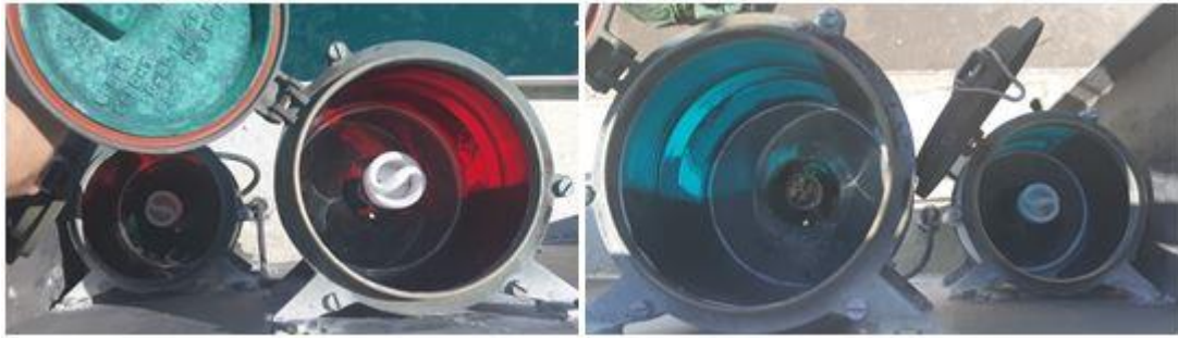
Figure 12 Navigational lights could not be shown to operate.
