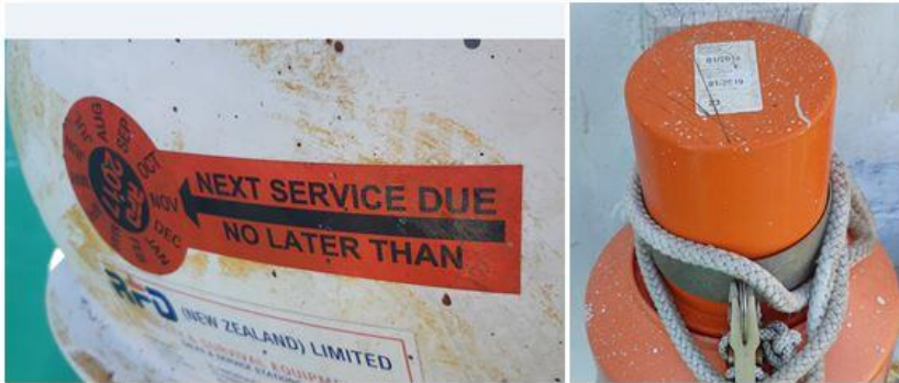
Figure 8 Liferaft and Lifebuoys expired.
