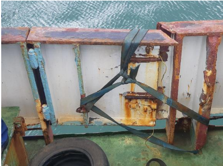
Figure 2 Access doors in bulwark not closing correctly.
