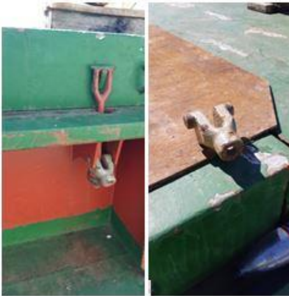
Figure 36 Cargo hatch securing dogs are not used by crew (rectified in inspection).
